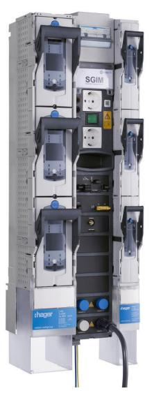
The SGIM is an easy-to-install measuring, monitoring and control system for digitizing of distribution substations and cable distribution cabinets in the smart grid. It enables cost-effective and uninterrupted installation in the 185mm busbar system in connection with NH striptype fuse-switch disconnectors in accordance with EN IEC 61439/60947 and thus the construction of a monitoring system at critical points and nodes in the distribution network.
